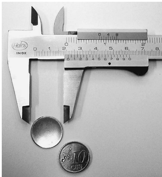
Fig. 6. Ag-doped bulk nanocrystalline titania specimens (2 cm diameter, 3 mm thickness).
